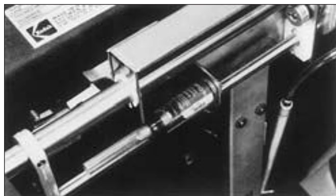
Snubbing paper carrier in an office copier.
