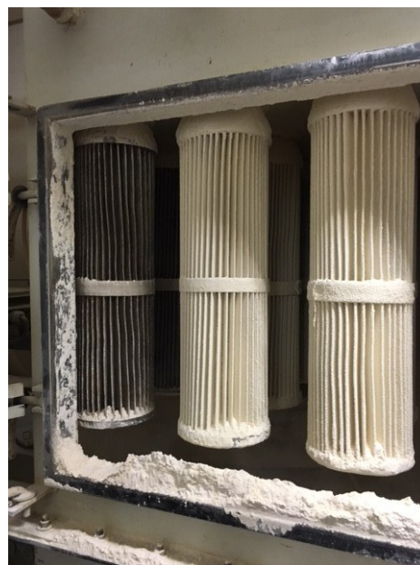
Filter left: Clearly less dust after pulsing
