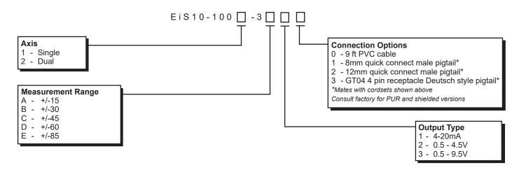
Ordering Example: EiS10-1001-3A10 Single Axis, +/-15 Range, 4-20mA, 9 ft. PVC cable.
