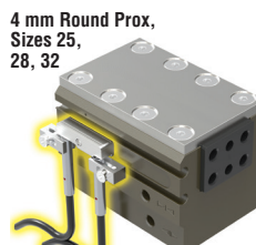
P - Inductive Proximity Switch (Includes -CP option, target, prox switch, and either one or two switch mounting brackets.) Target comes unassembled.
