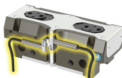
P - Inductive Proximity Switch (Includes target, one or two switch mounting brackets, and 8 mm threaded proximity switch, or switches, depending on code.) Target comes assembled in unit.
