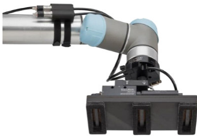
Custom vacuum gripper with manifold mounted venturi vacuum pump, .24 kg
