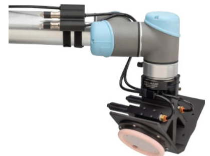
Dual head vacuum gripper for grinding flash from molded silicone parts. Weight: .46 kg
