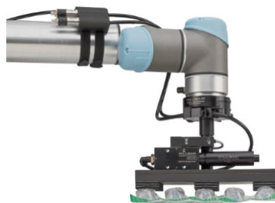
Handling packaged hypodermic needles for in-the-box packaging
